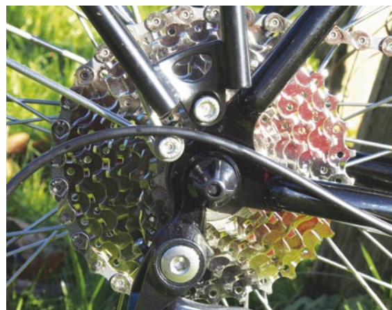
Above Carrier wants and gets a bigger (M6) bolt
